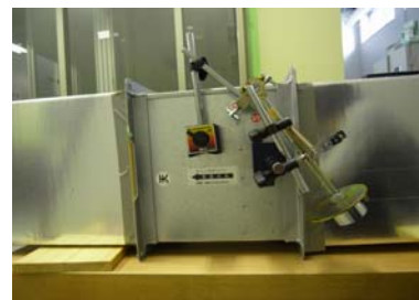
Photo 1: Improved backdraft damper
