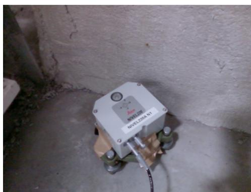
**Figure 7 Inclination sensor-NIVEL 220 on site.**
