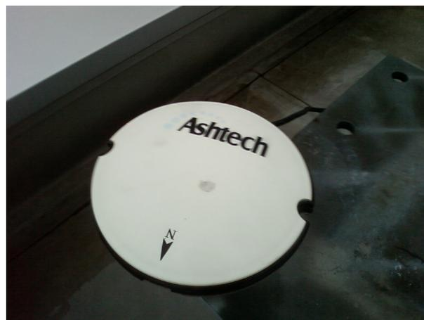
**Figure 1 Rover GPS on top of Yokohama Island Tower**
