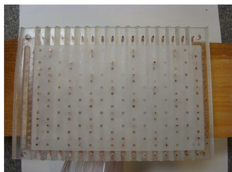
(b) Close-up view of a porous roof cover sheet
