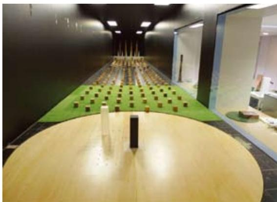
Figure 1. Experimental models in wind tunnel
