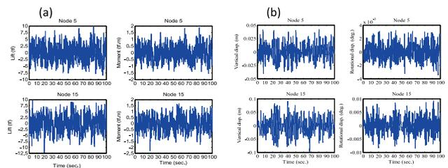
Fig.8 Time series of global forces (a) and global response (b) of nodes 5 & 15 at mean velocity  $U=20\text{m/s}$
