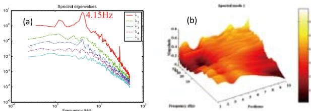
Fig.6 First five spectral eigenvalues and first spectral mode
