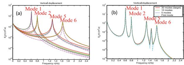
Fig.7 Power spectra of generalized (a) and global responses (b) of vertical displacement
