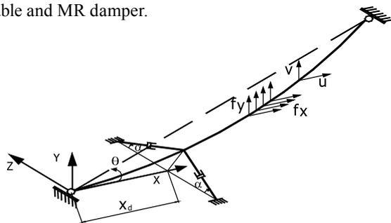
Fig. 4 Mathematic model of cable with attached damper
