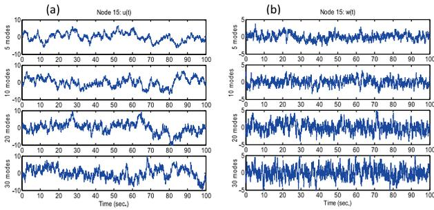
Fig.3 Simulated time series of fluctuating wind speeds  $u$  (a) and  $w$  (b) at  $U=20\text{m/s}$  (Node 15)
