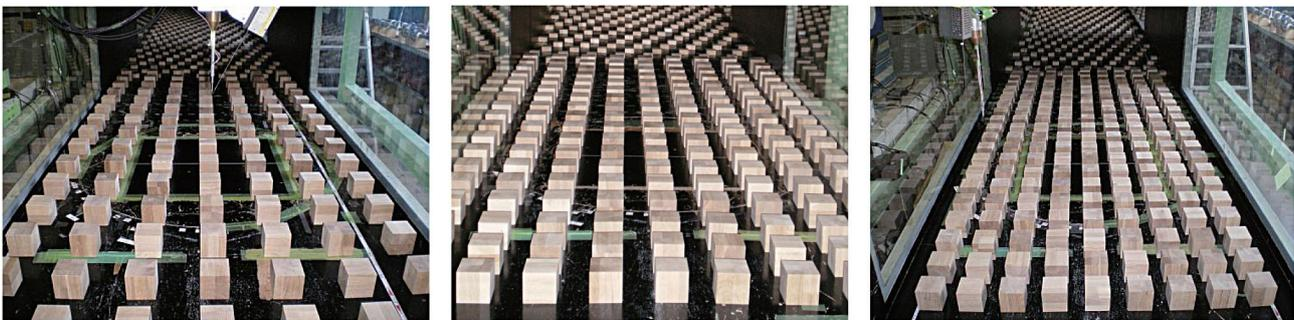
Figure 1: Idealised urban canopies with uniform building height and 16% (left), 25% (centre), and 34% (right) building coverage ratio.
