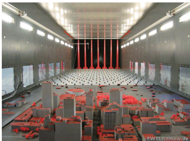
Figure 3. The 1:300 scale model of the Central Business District of Oklahoma City, mounted in the test section of the large boundary layer wind tunnel at EWTL.
