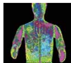
Figure 5. Infrared image on thermal mannequin in cross-ventilated environment
