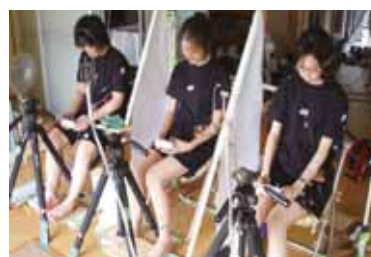
Figure 4. Field experiment on thermal comfort in cross-ventilated environment
