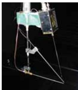
Figure 8: System for simultaneously measuring fluctuating concentration, velocity and temperature
