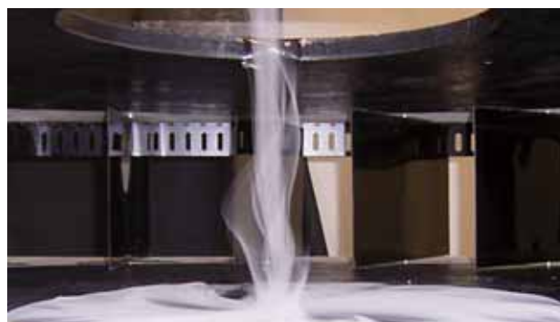
Figure 3 Flow visualization of tornado-like flow
