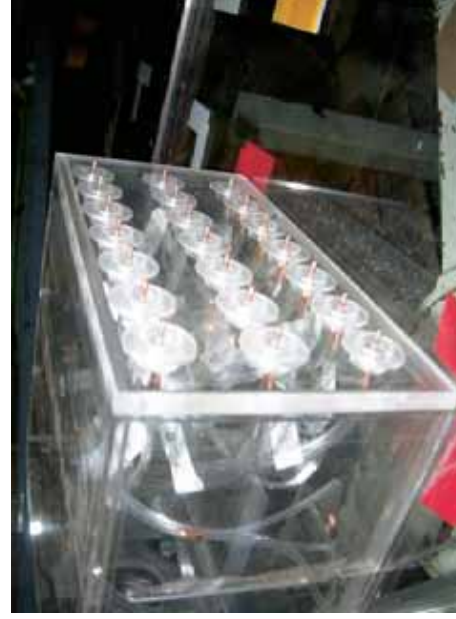
Photo 1. Irwin's surface wind sensors placed on wall surface
