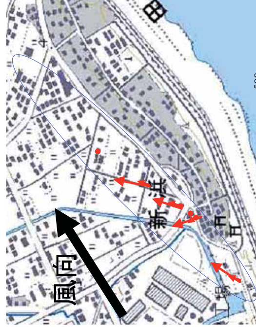
Figure 6. Damage situation (The vector shows the flying direction of the tilt)
