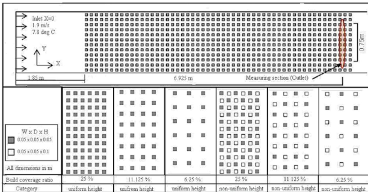
Figure 6 Experimental setup and List of experimental cases
