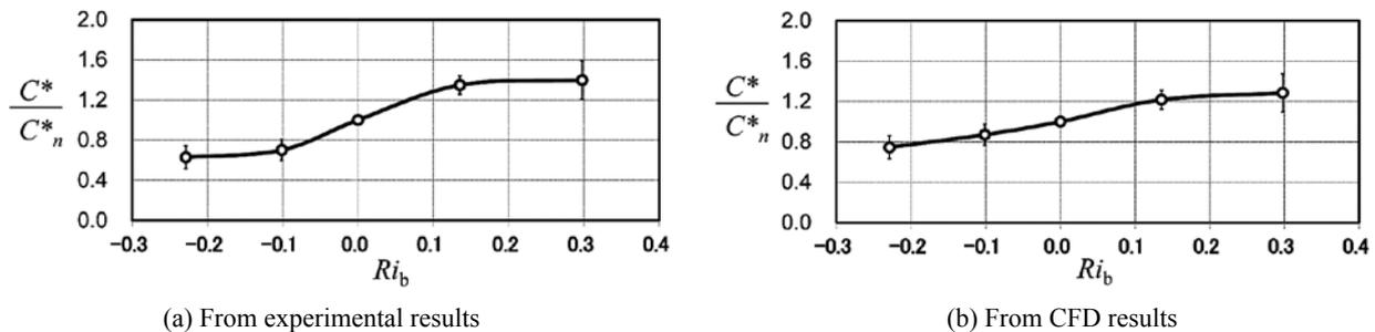
Figure 15 Stability Effect Ratio (SER) = Ratio between  $C^*$  under un-neutral condition and  $C^*_n$  under neutral condition
