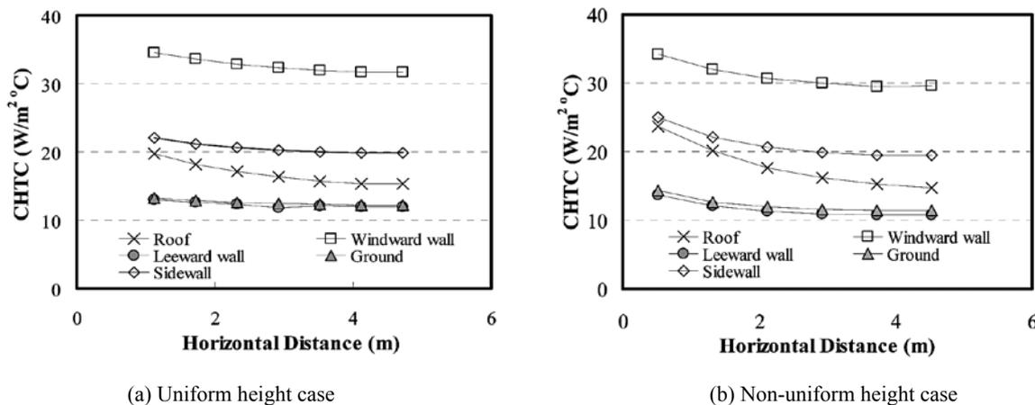
Figure 8 CHTC profile in horizontal distance in the flow direction for individual canopy surfaces for 6% BCR
