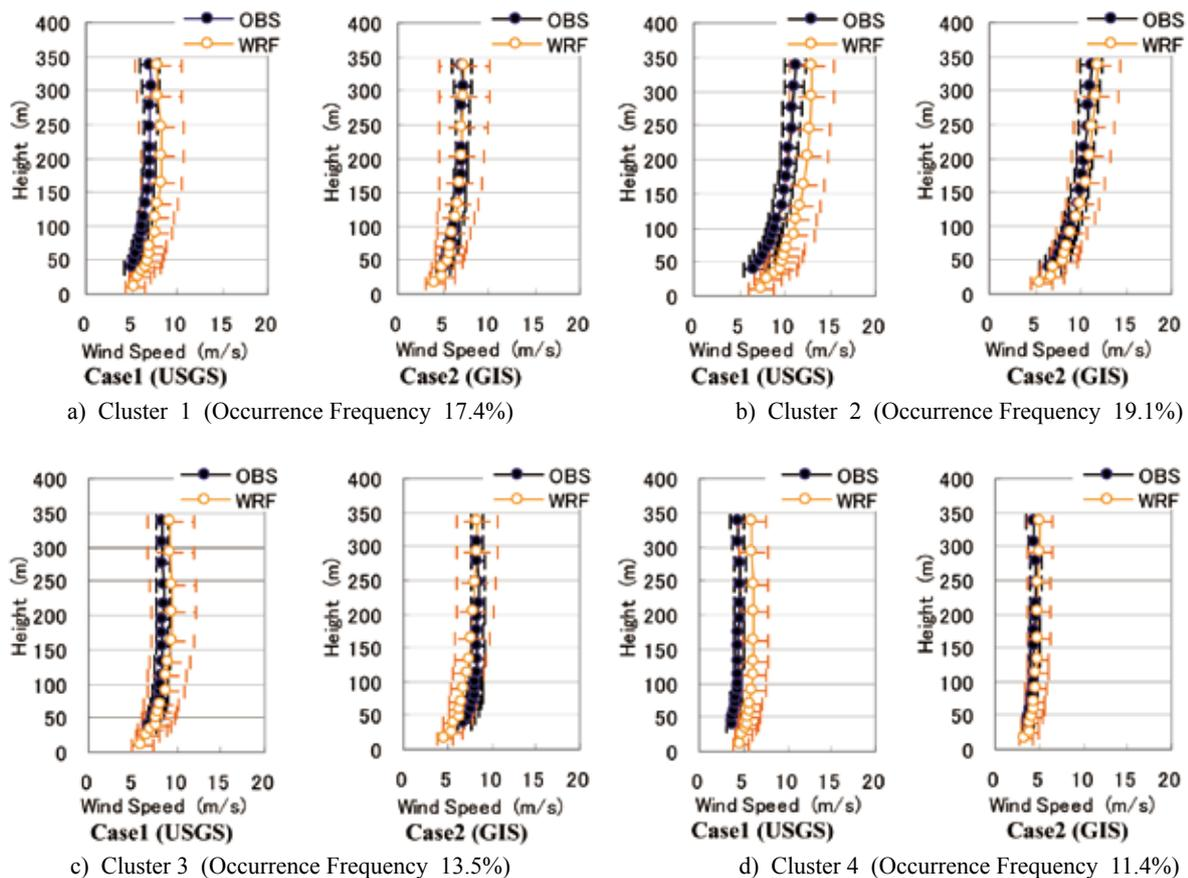
Figure 5 Vertical Profile of Mean Wind Speed
