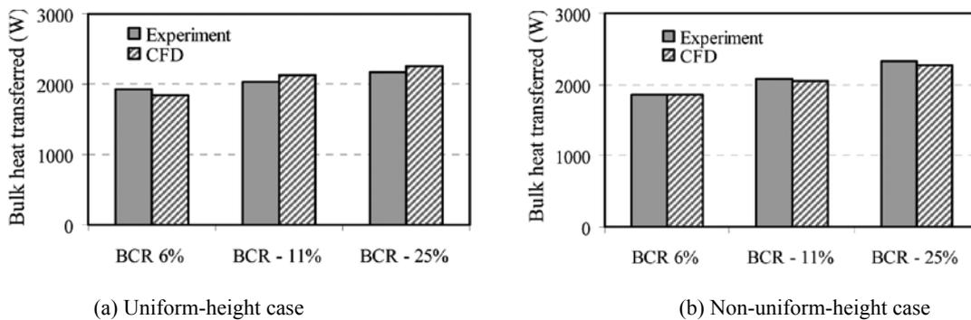
Figure 7 Comparison between experiment and CFD simulations: Bulk heat transferred from urban canopy for various BCR
