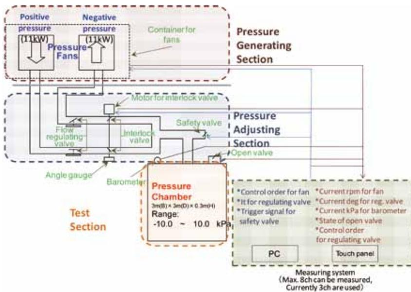
Figure 3 Conceptual Drawing of experimental system
