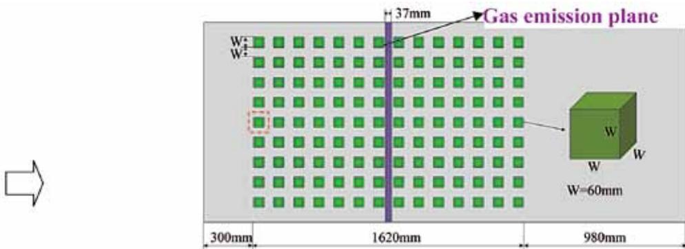
Figure 12 Arrangement of building blocks
