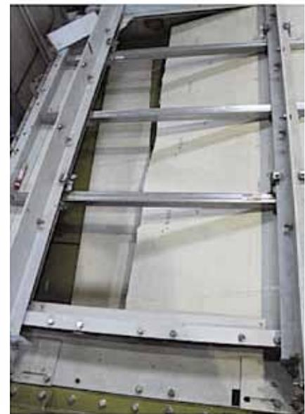
Figure 4 Example of specimen (after loading extraordinary pressure)
