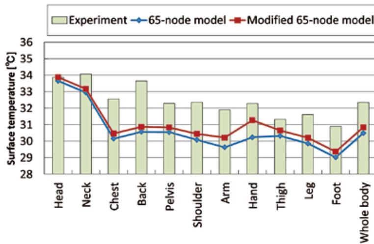
Figure 5 Prediction accuracy of body skin temperatures at 32°C in early summer environment by modified 65-node model
