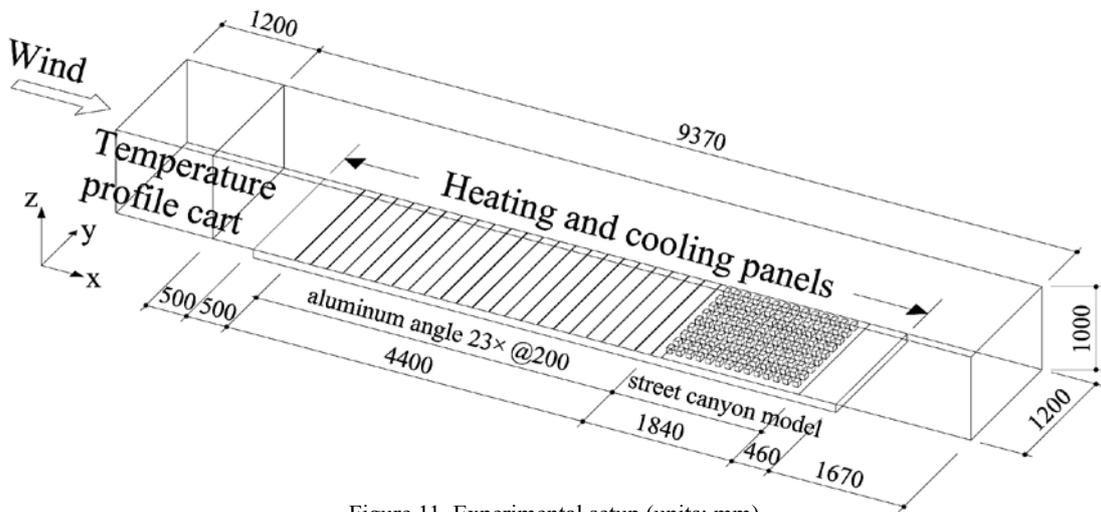
Figure 11 Experimental setup (units: mm)
