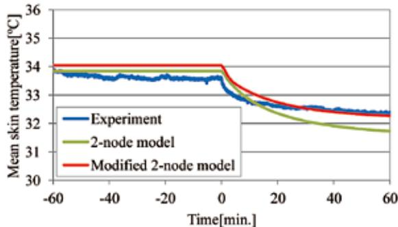
Figure 3 Comparison of measured and predicted skin temperatures in cross-ventilated environment
