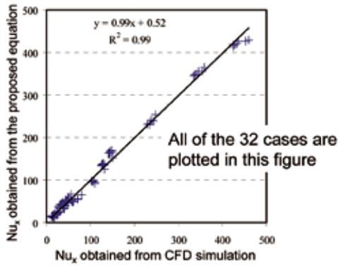
Figure 9 Comparison between local Nusselt number obtained from CFD simulation and proposed equation
