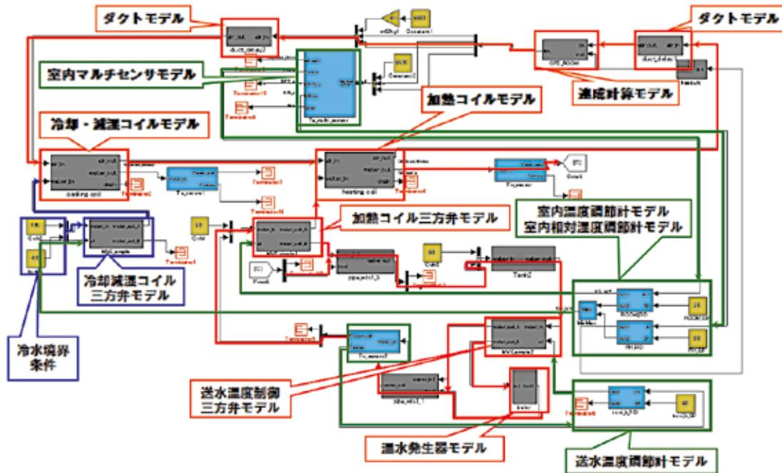
Figure 9 Coupled dynamic system model
