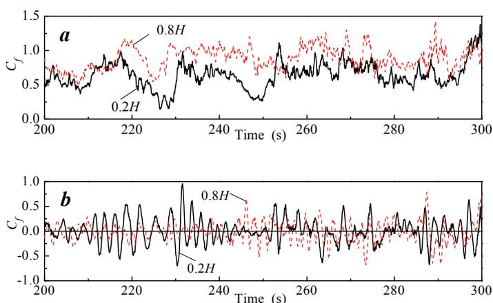
Figure 3. Overall wind force coefficients: (a) along-wind force coefficient; (b) across-wind force coefficient
