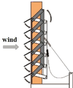
Figure 5. Mechanism of the natural ventilation system
