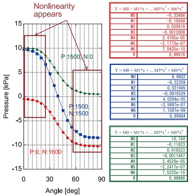
Figure 5. Static relationship between angle of interlock valve and chamber pressure
