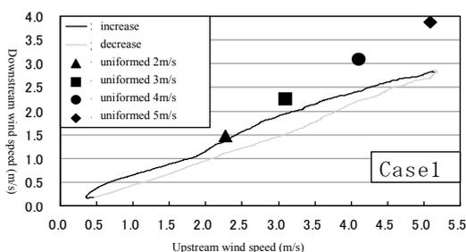
Figure 7. Relation between downstream wind speed and upstream wind speed
