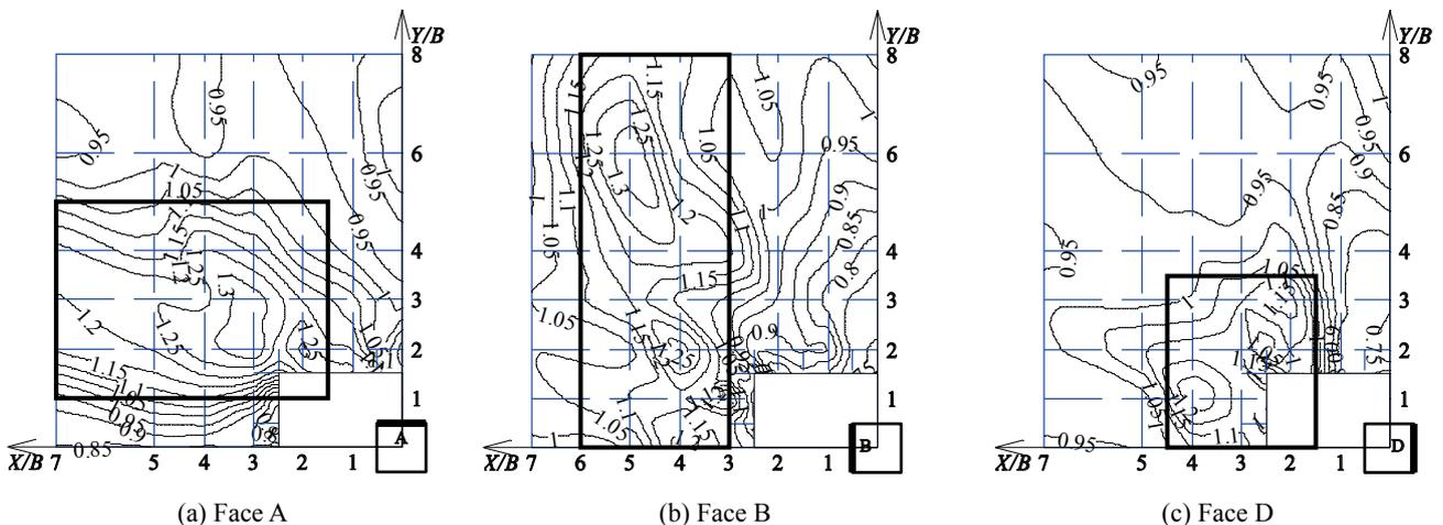
Figure 3. Contour of interference factor for negative peak pressure on wall A, B, and D
