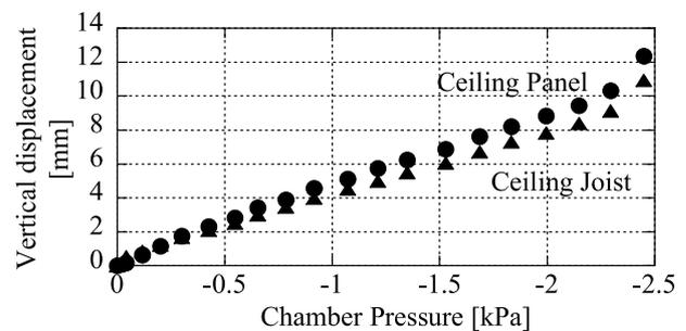
Figure 7. Vertical displacement of Ceiling Panel and Ceiling Joist
