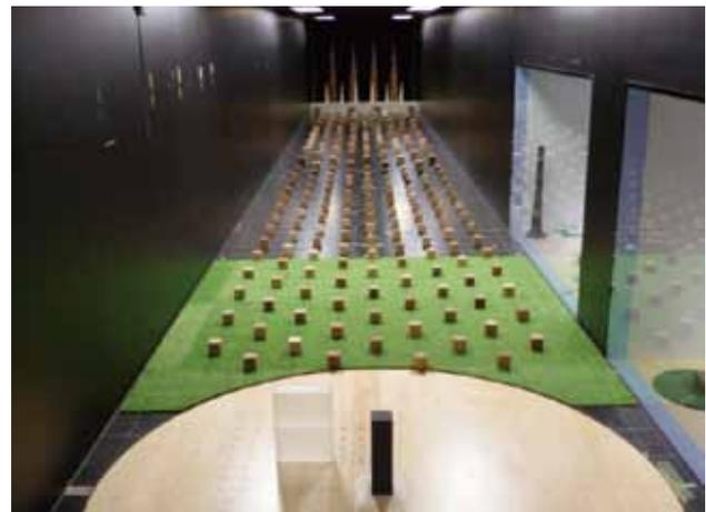
Figure 2. Experimental setup in wind tunnel
