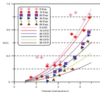
Figure 6. Wind force on wings
