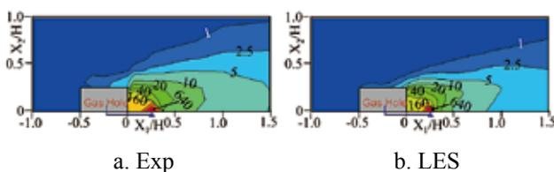
Figure 7. Horizontal distributions of mean concentration  $\langle c \rangle / C_0$  ( $X_y/H=0.025$ ).
