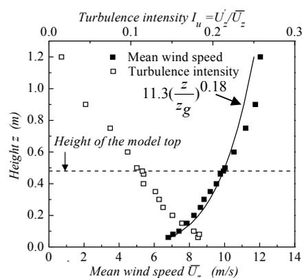
Figure 2. Mean wind speed and turbulence intensity profiles
