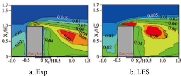
Figure 5. Distributions of turbulent kinetic energy  $k/U_H^2$
