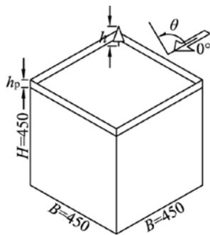
Figure 9. Dimensions of model of tree and building
