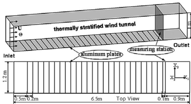
a. Precursor simulation domain and roughness elements arrangement
