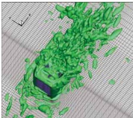
Figure 6. Instantaneous vortex structures (LES,  $Q=200 \text{ s}^{-1}$ )
