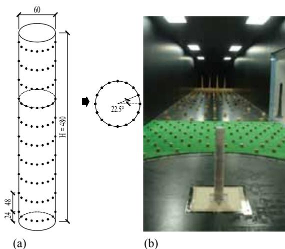
Figure 1. Wind pressure test model: (a) configuration of test model (unit: mm); (b) model in wind tunnel
