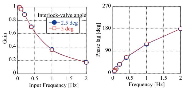
Figure 6. Gain and Phase lag of pressure chamber (2.5 deg and 5.0 deg)
