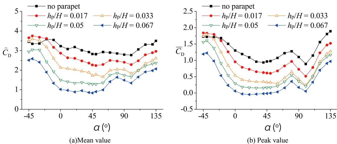
Figure 11. Effect of parape height ( $h_p$  is parape height)
