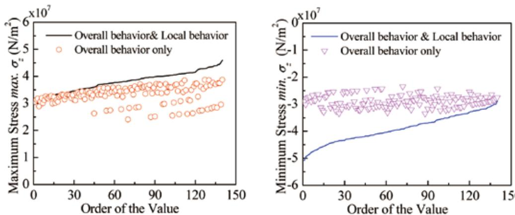
Figure 5. Comparison of maximum and minimum axial normal stresses according to order of values
