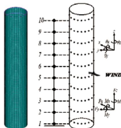
Figure 4. FE model and lumped-mass model system
