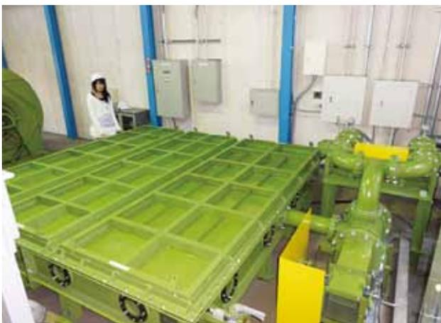
Figure 4. Test facility (LEFT: Open-topped pressure chamber,RIGHT: Pressure adjustment mechanism)
