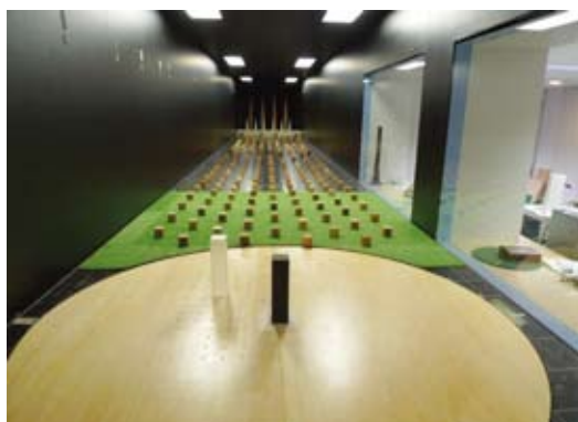
Figure 1. Experimental models in wind tunnel
