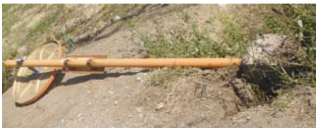
Fig.12. Sign pole uprooted in tornado's path
