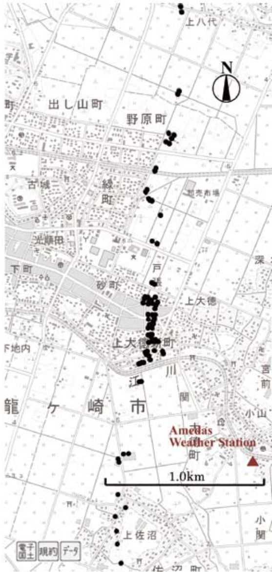
Fig. 9 Distribution of damage due to tornado (●)
