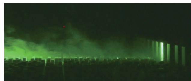
Figure 3. Visualization of “vertical ventilation paths” behind coastal high-rise buildings.
