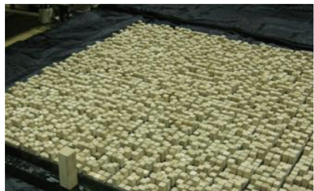
Figure 2. Wind tunnel experiment for coastal city in Tokyo.
